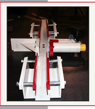
Stringer-Mate Stringer Splicers are designed to increase the yield of any pallet recycling operation.
