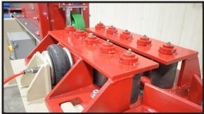
The Pallet Doctor Stringer Sizer machines are designed specifically for pallet recycling. The Sizer utilizes a special nail cutting cutter head to easily cut through both the stringers and nails to provide a consistent, high quality product.
